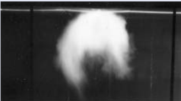
Fig. 2: Without Varyset, \dot{V} = 11 l/s; \Delta t = -8 K
