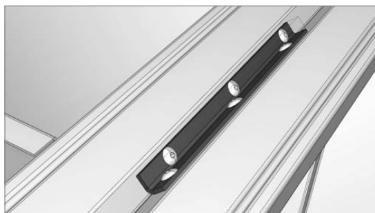
Fgi. 5: Rivet on the angle brackets
