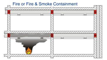
Fire Damper - To maintain COMPARTMENTATION **CLOSE & remain closed**  Maintain fire (& smoke) integrity of the support construction
